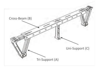
You will need 2 screws per Cross-Beam, 2 per Tri-Support and 2 per Uni-Support. We recommend 4 x 40mm (8 x  $1\frac{1}{2}$ ") wood screws. You will also need the same size screws to fix the loft boards on to the Cross-Beams.
